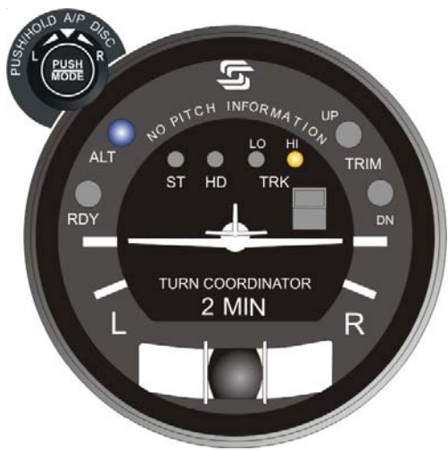
Fig. 2-25. AP Display, HI TRK and ALT HOLD Modes Engaged (System Thirty)
