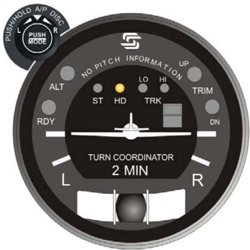
Fig. 2-22. AP Display, HD Mode Engaged (System Thirty)
