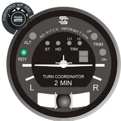
Fig. 2-3. AP Display, RDY for Operation (System Twenty)
