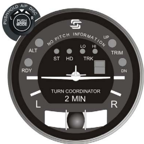
Fig. 2-4. AP Display, Turn Coordinator Failure (System Twenty)
