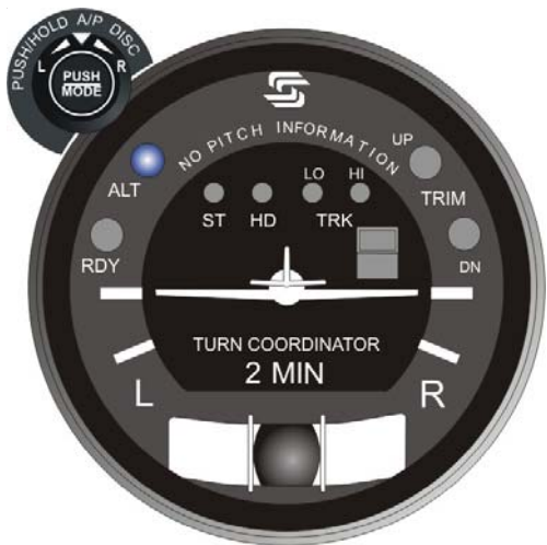
Fig. 2-8. AP Display, ALT Lamp Only Illuminated (System Thirty)
