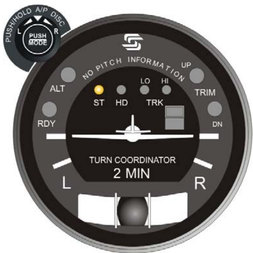
Fig. 2-17. AP Display, ST Mode Engaged (System Twenty)
