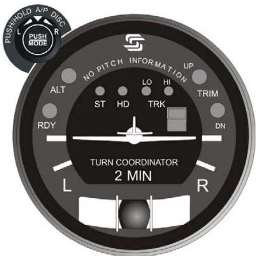
Fig. 2-9. AP Display, All Lamps Extinguished (System Thirty)
