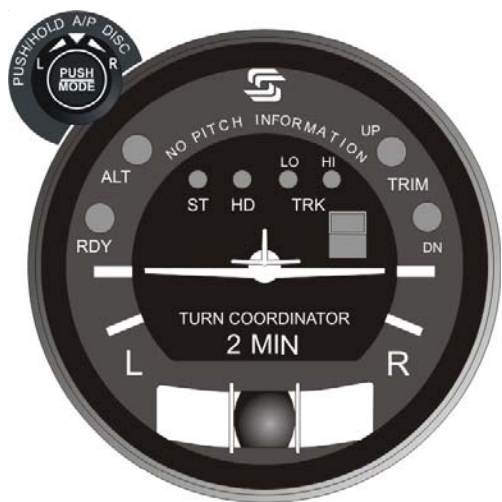
Fig. 2-11. AP Display, Turn Coordinator Failure (System Thirty)
