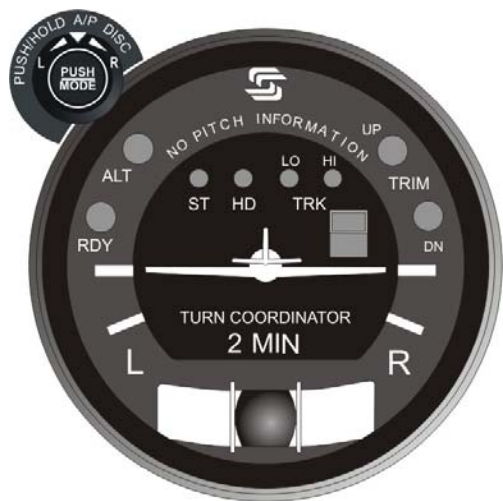
Fig. 2-2. AP Display, All Lamps Extinguished (System Twenty)
