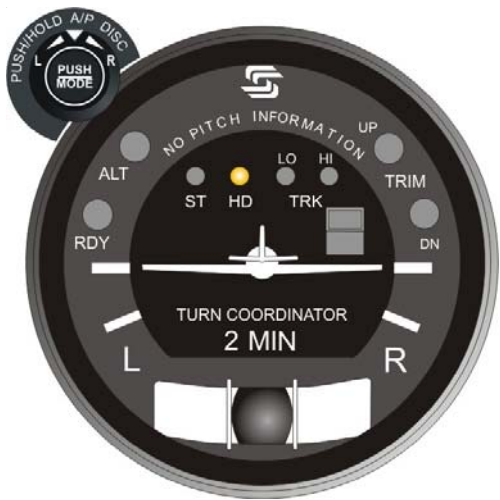
Fig. 2-18. AP Display, HD Mode Engaged (System Twenty)
